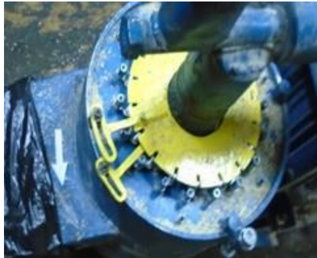
Fig. 3. Mechanism of synchronous rotation of knives
